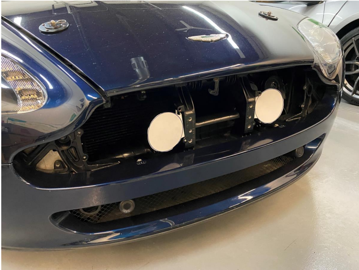
#3 Experiment with Carboard Mockup to place lights – they seem to fit perfectly on center structure
